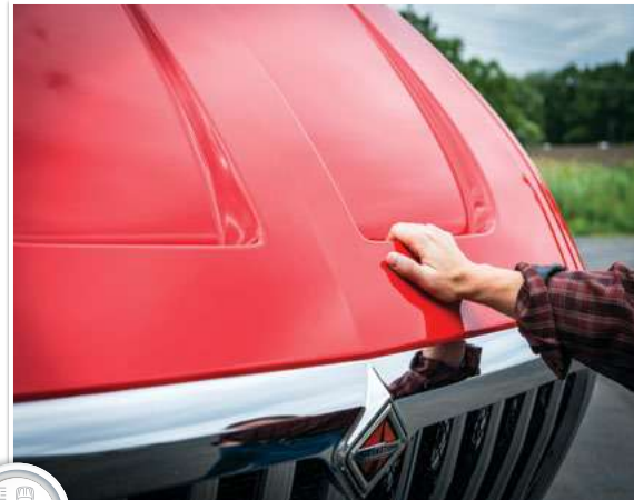
FORWARD-TILTING HOOD IS EASY TO OPEN
